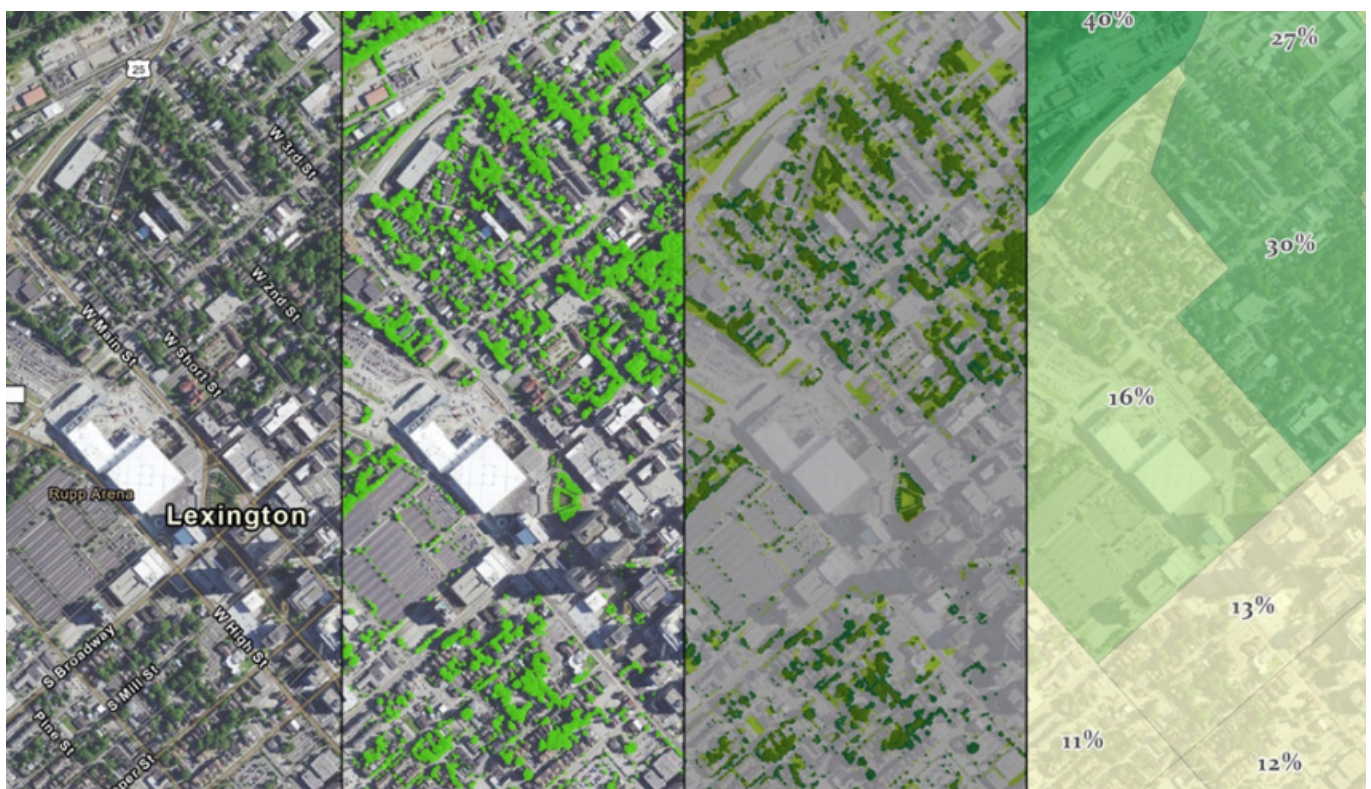
Figure 1. Aerial imagery of downtown Lexington, Kentucky (left), the derived land cover classification raster (center), and percent canopy cover summarized by census block groups (right).
