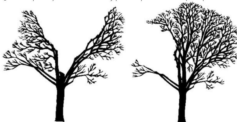
Figure 38. Examples of trees directionally pruned for clearance from power lines
